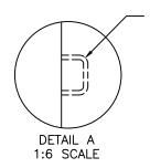
TETHERING LOOPS ON ENDS ARE CENTERED FROM FRONT TO BACK. TETHERING LOOPS ON BACK ARE LOCATED 12" FROM EACH END.
